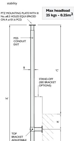
OPTION OF INTERNAL **CABLING THROUGH BOTTOM BRACKET**
