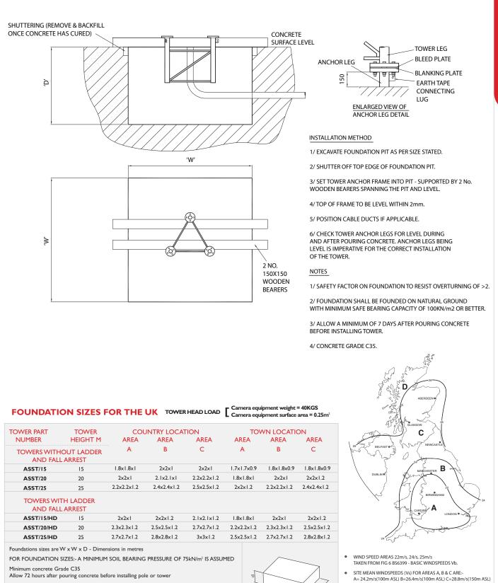
Allow 72 hours after pouring concrete before installing pole or tower
