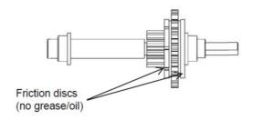
Apply a drop or two of #30 weight engine oil to each bushing I.D. and to the ratchet pawl pivot points. Maintain a thin layer of chassis grease on the gear teeth.
