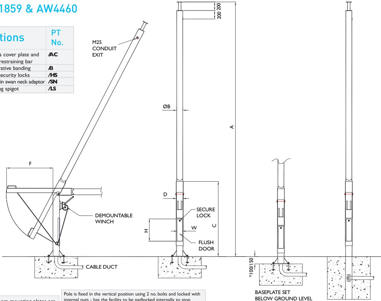
All camera mounting plates are Ø 127 with 8 No Ø 8.5 equi-spaced on 101.6 PCD. Ø 40 thro' column spacer
