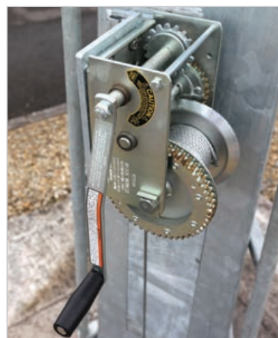
DW2500 Winch mounted on ANCT tower. This bracket type for ANCT towers only.
