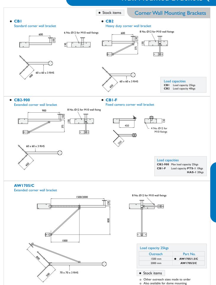
All brackets for camera mounting have a Ø127 mounting plate with Ø8.5 holes equi - spaced on 101.6 PCD
