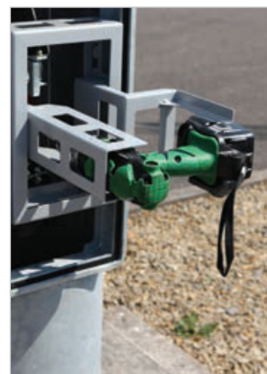
DSB - Drill Support Bracket, with Drill winder located in bracket
