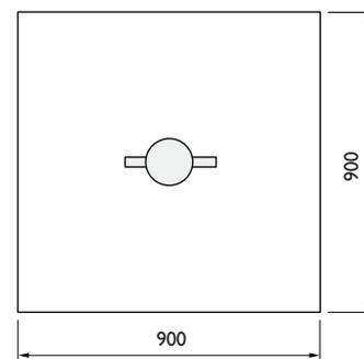
Set bollard into foundation. Fill bollard with concrete - capping plate has rags on underside to push into the concrete filled bollard holding plate in position once concrete has set
