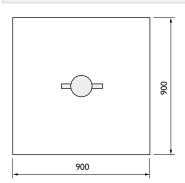
Set bollard into foundation. Fill bollard with concrete - capping plate has rags on underside to push into the concrete  $\dot{\text{filled bollard holding plate in position} } \\$ once concrete has set
