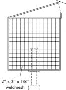
Padlockable hinged door to enable access to camera equipment for servicing is available as an option
