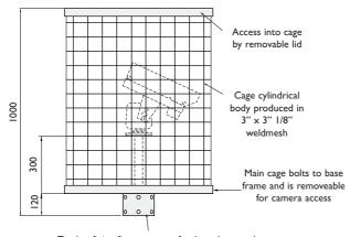
Top hat fixing fits over top of pole and secured with 6No. bolts. Size made to suit pole diameter
