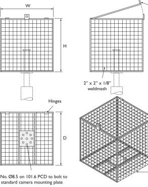
Padlockable hinged door to enable access to camera equipment for servicing is available as an option
