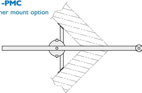
All brackets for camera mounting have a Ø127 mounting plate with 8 no Ø8.5 equi - spaced on 101.6 PCD
