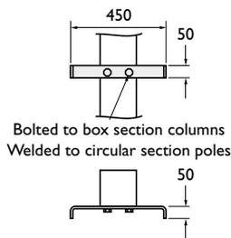
Bolted to box section columns
