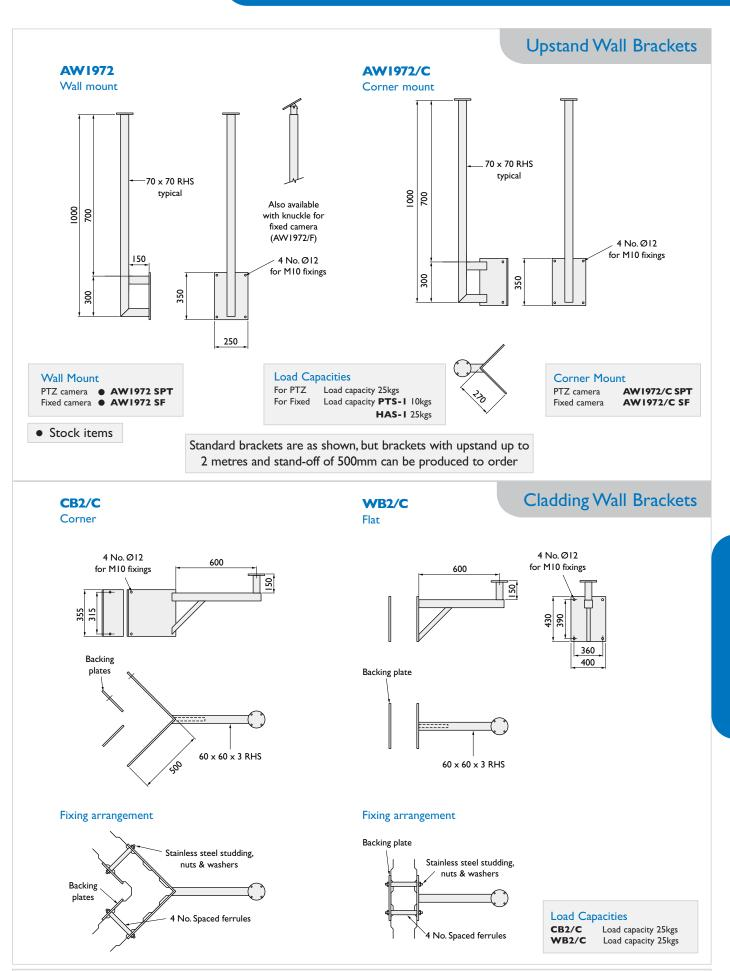
All brackets for camera mounting have a Ø127 mounting plate with 8 no Ø8.5 equi - spaced on 101.6 PCD
