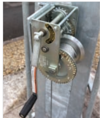
DW2500 Winch mounted on ANCT tower. This bracket type for ANCT towers only.
